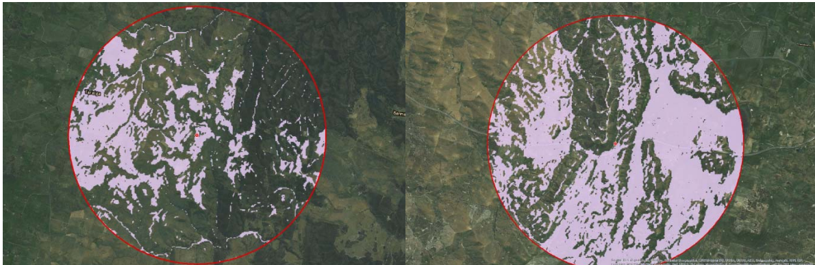
Figure 58 Example ranking results for Taralga (left) and Cullerin Range (right) wind farms (available solar farm area is shaded)
