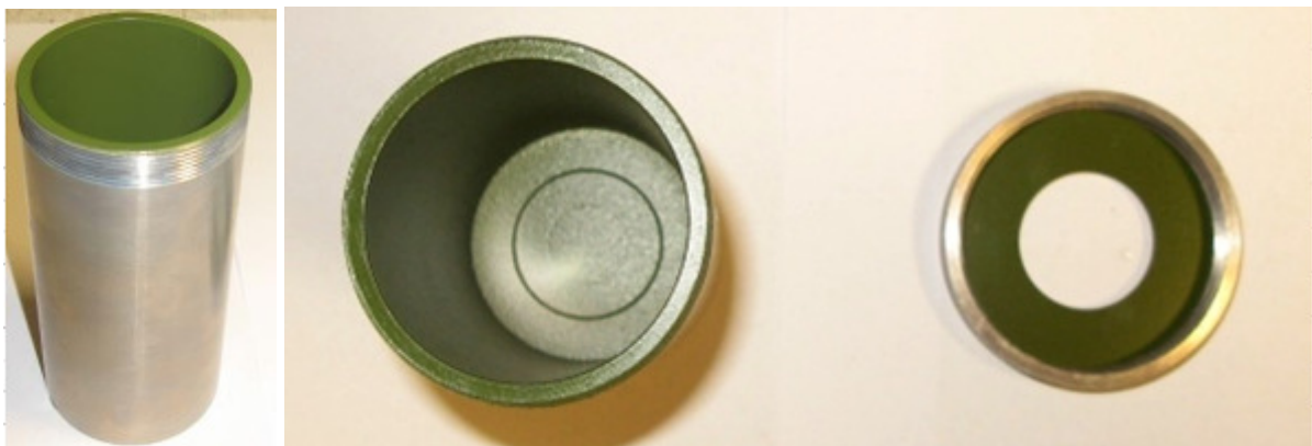
Plate 2: The new Aluminium Bottle, partly coated with PTFE.
