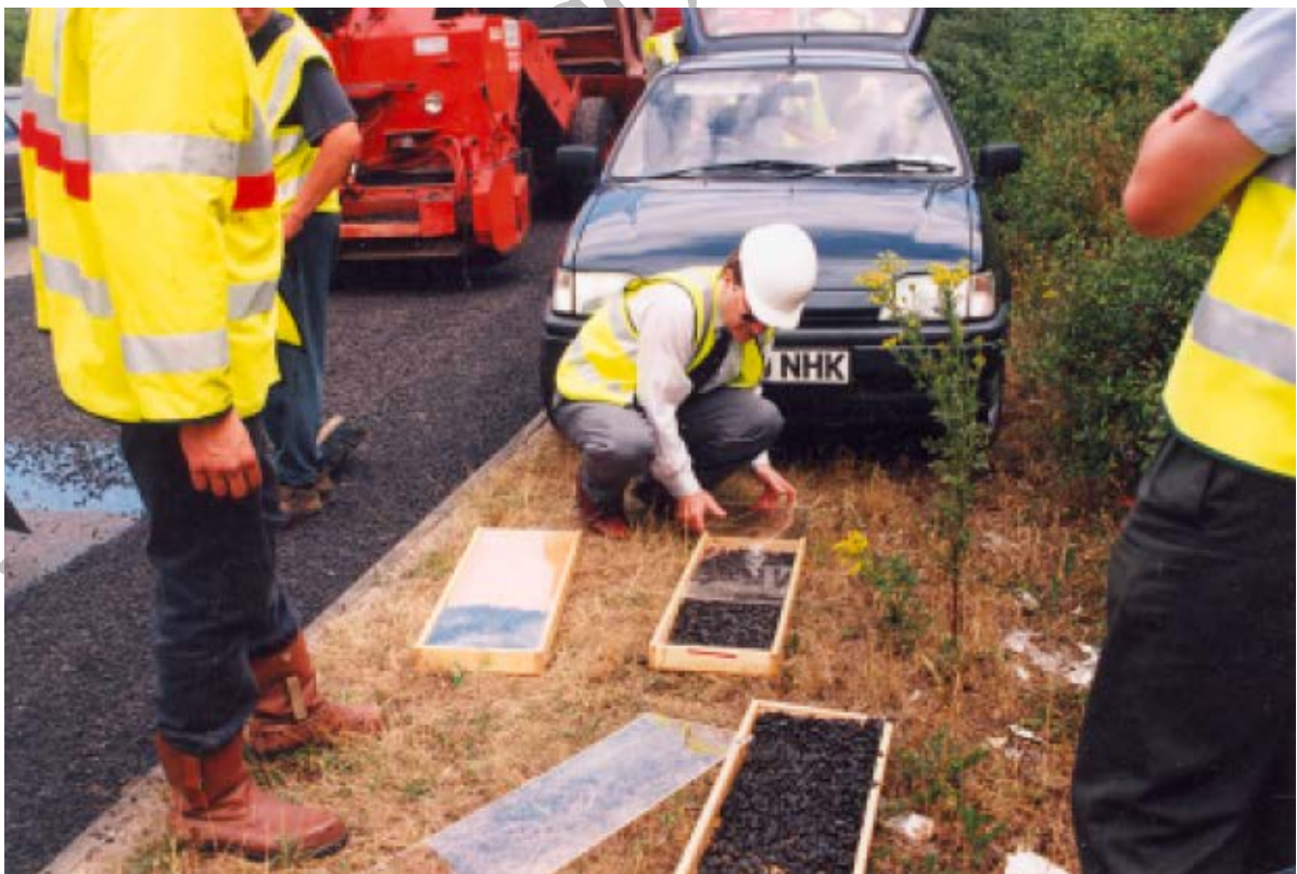
Figure 8.18 Fitting the Clear Calibrated Sleeve Tops to the Chipping Rate of Spread Boxes
