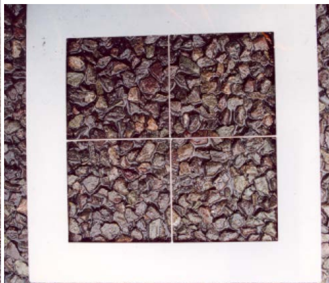
Inverted Double Dressing Age 15 years, Surface Comprising 14mm Chippings (No Loss)
