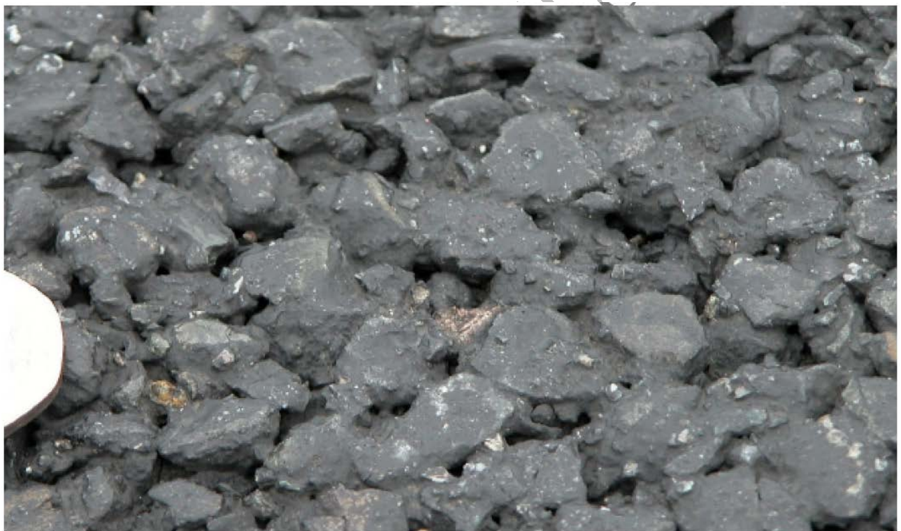
Figure 4.5 Close-up of 0/10mm TASC, One Year after Laying, Showing How the Surface Film of Binder is Wearing Off to Reveal the Micro-texture. Aggregate Particles are Held by the Polymer Modified Binder and They Contribute to the Overall Skid Resistance.
