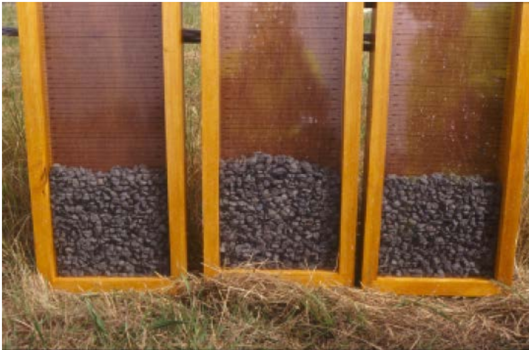
Figure 8.19 Measuring the Rate of Spread of Chippings in Terms of Bulk Volume
