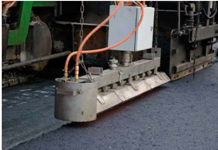
Figure 12.29 Example of an Infra-red Joint Heater, which Automatically Cuts Out when Paver Stops
