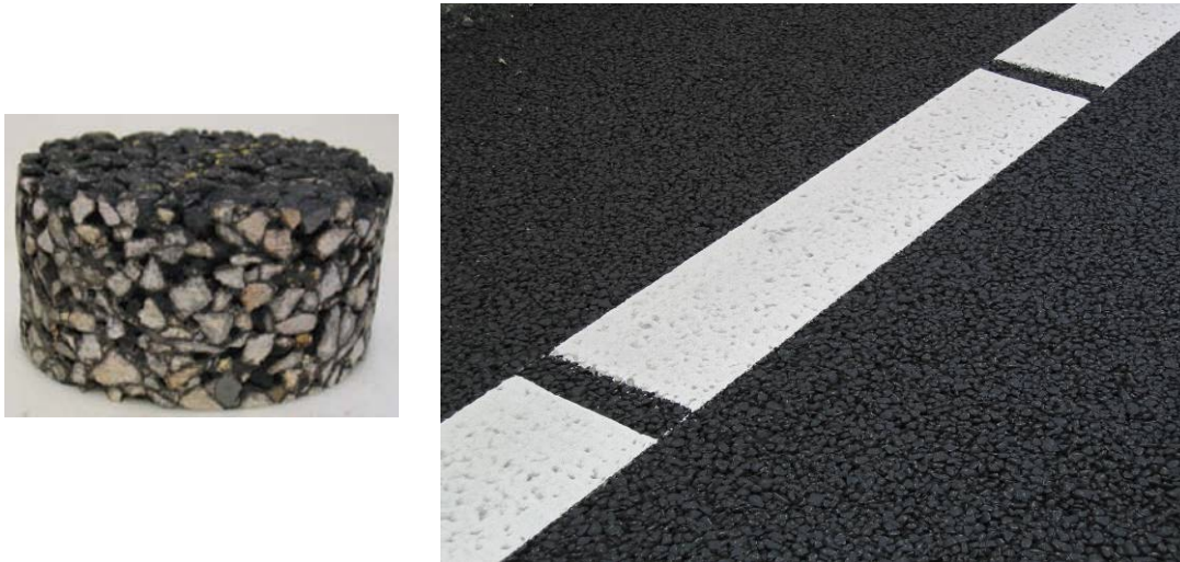
Figure 7. 2 Typical Porous Asphalt Material (Source: URS and EAPA)
