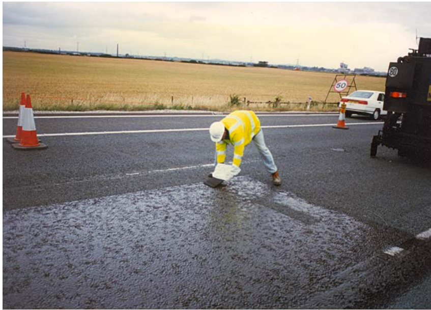
Figure 12.25 Rate of Spread of Bond Coat Carpet Tile Test (EN12272-1)
