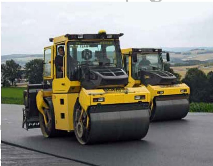
Figure 12.38 Rollers with Density and Temperature Monitoring and GPS Location
