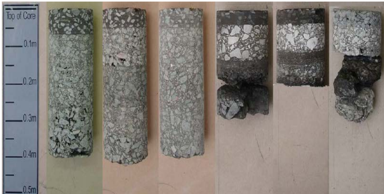
Figure 2.1 Illustration of Different Pavement Materials and Thicknesses
