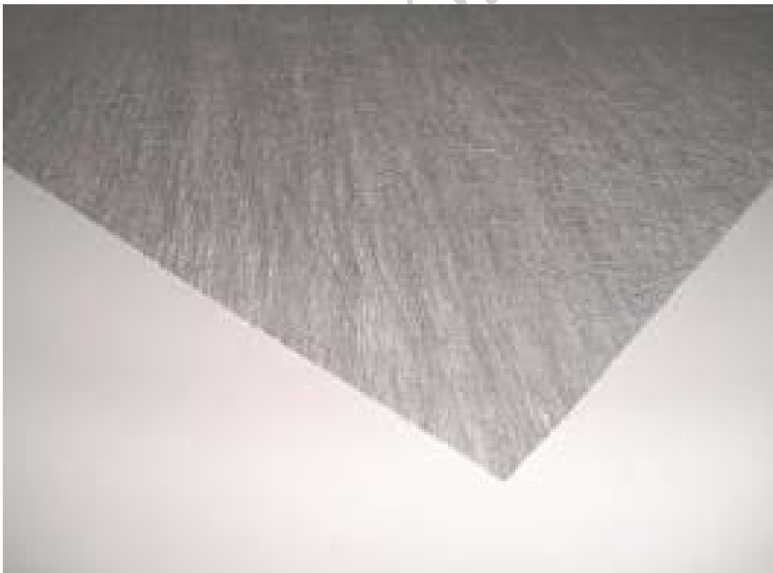
Figure 11.5: Non-woven Fabrics (typically Needle Punched Polypropylene but Polyester and Combinations using Glass Fibres are also Available).
