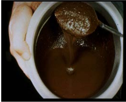
Figure 10.14 Slurry Surfacing Consistency – Fluid Brown Unbroken Emulsion Mixture whilst Agitated
