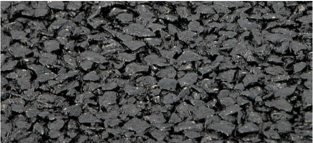
Figure 4.4 Negative Macro-texture of a Freshly Laid Polymer Modified 0/10mm TASC
