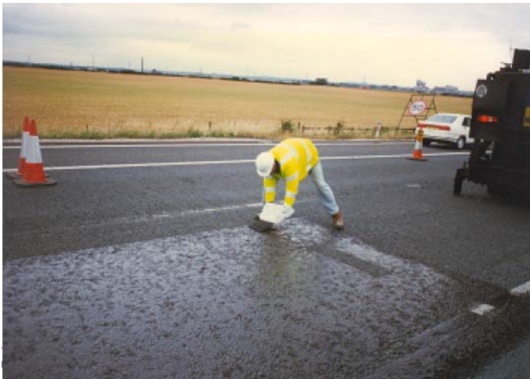
Figure 8.16 Rate of Spread of Binder Test, Note the Use of a Plastic Bag to Collect the 250 mm Square Carpet Tile
