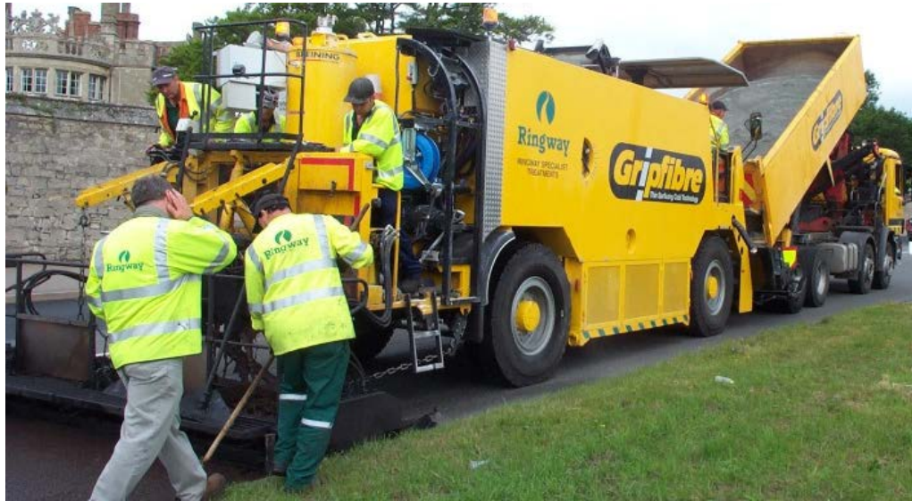
Figure 10.12 Front Loading Microsurfacing Machine
