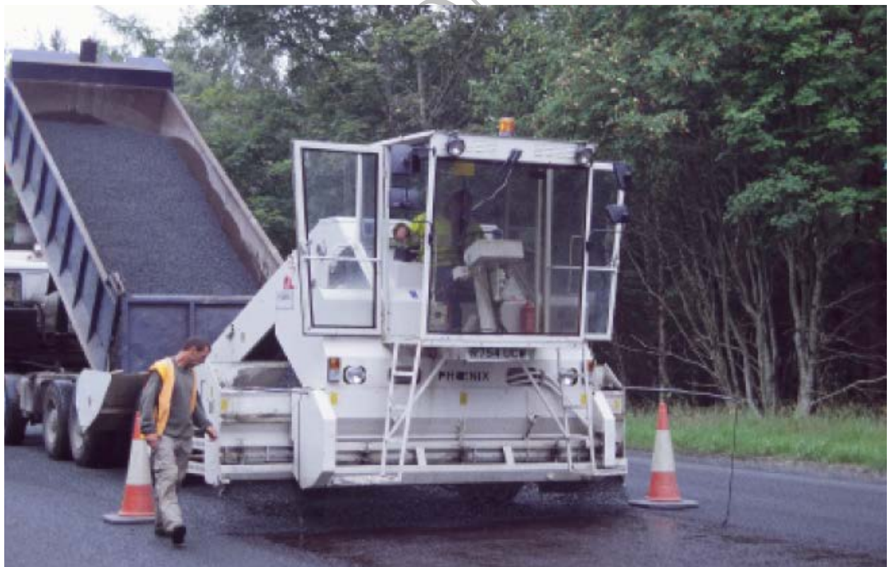
Figure 8.5 14mm Chippings Applied with a Truly Variable Phoenix Gritting Machine
