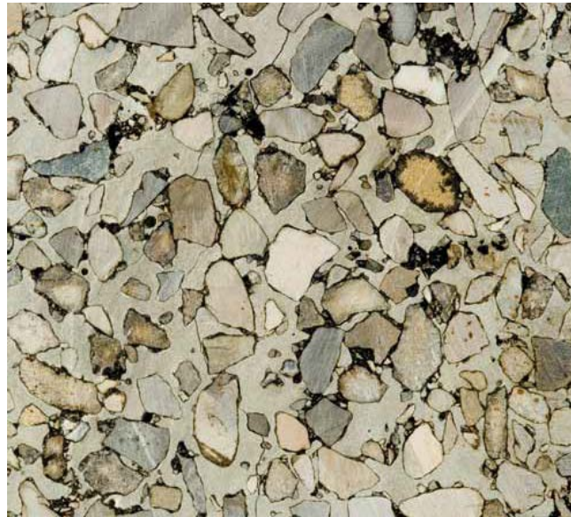
Figure 13.13 Cement Grouted Porous Asphalt Cross-section
