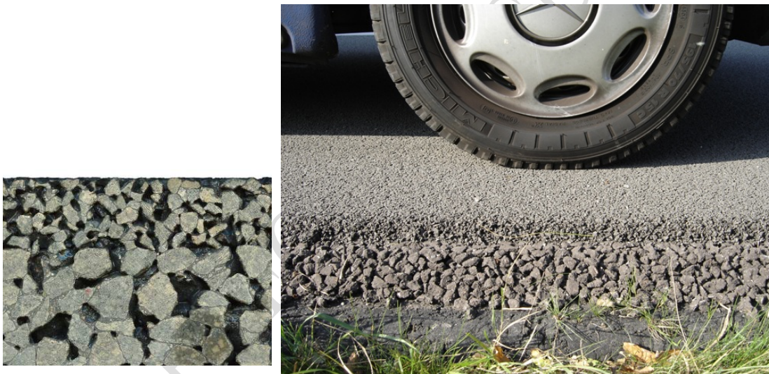
Figure 7. 2 Typical Porous Asphalt Material (Source: URS and EAPA)
