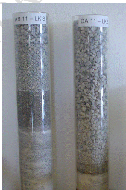
Figure 7. 1 Typical Porous Asphalt Grading on the Right Compared with the Continuous Grading of an Asphalt Surface Course on the Left
