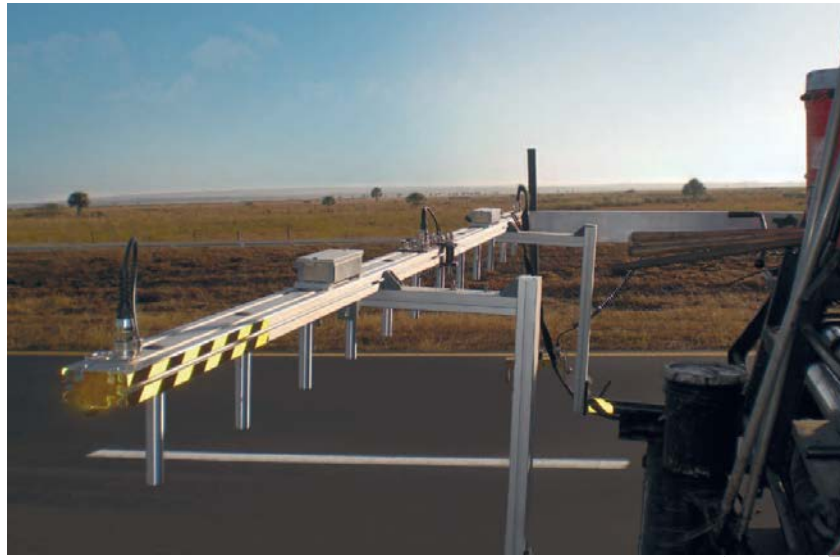
Figure 12.34 Infra-red Detectors to Monitor Heat from Paved Asphalt
