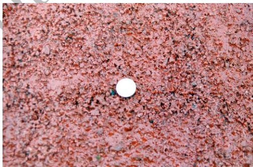
Figure 13.4 Loss of Colour after Two Years in Service (Thermosetting Resin System)
