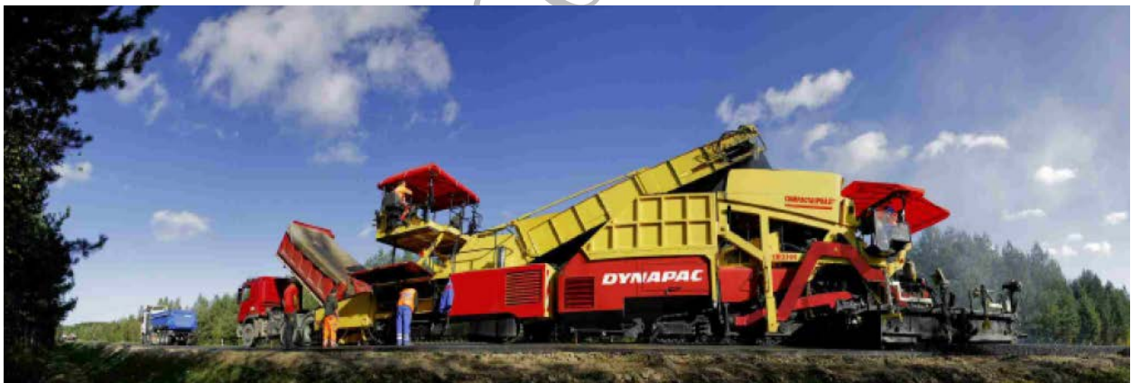
Figure 12.2 Dual Laying Paver (Compact Asphalt Paver) with Separate Feeds
