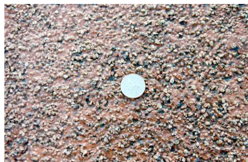
Figure 13.4 Loss of Colour after Two Years in Service (Thermosetting Resin System)
