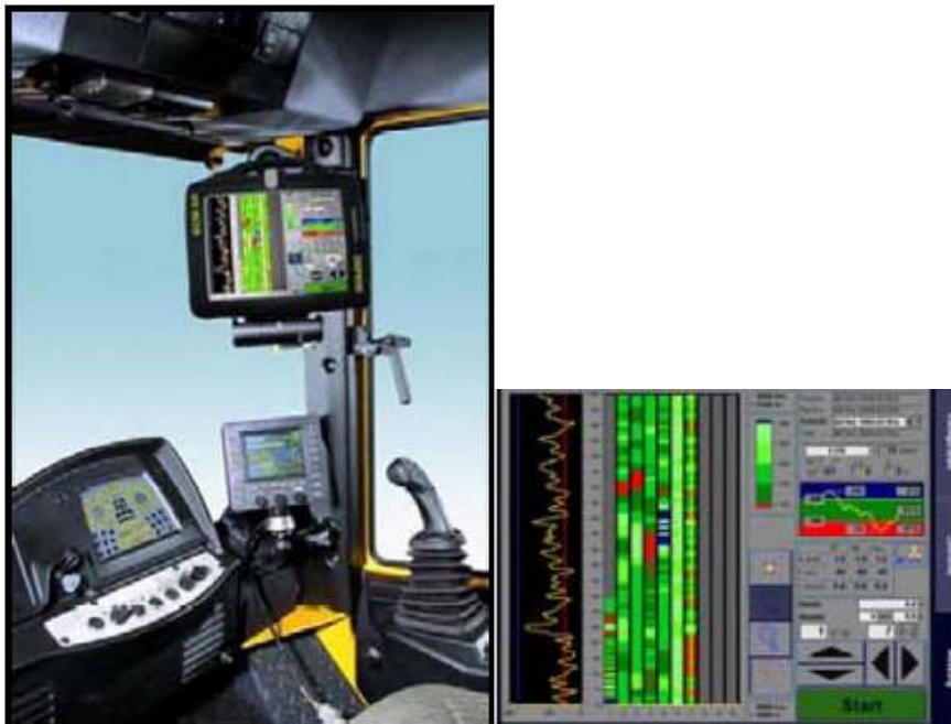
Figure 12.39 Monitor Output in Roller Cab to Indicate Areas of Low Density and Low Temperature
