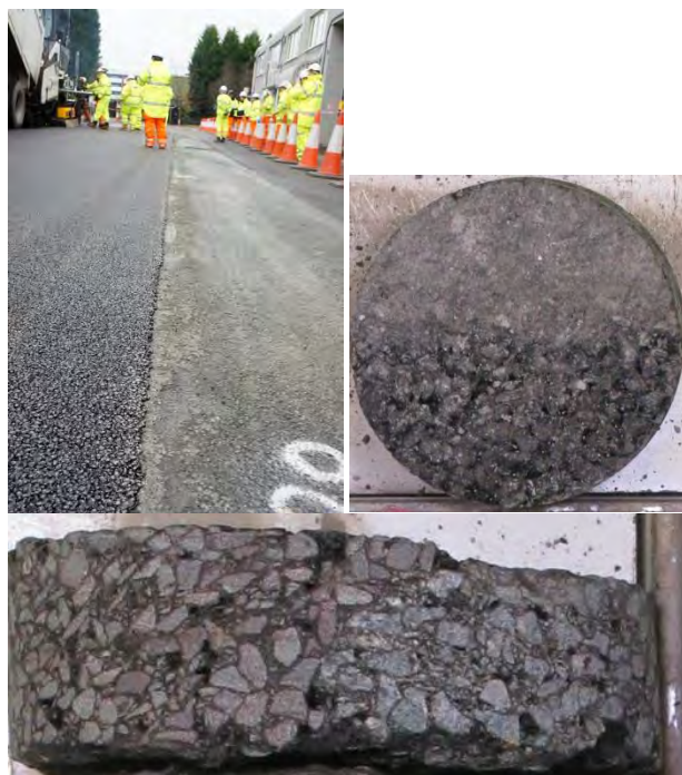
Figure 15: i) Photograph of the joint ii) Core 43 surface iii) Core 43 profile
