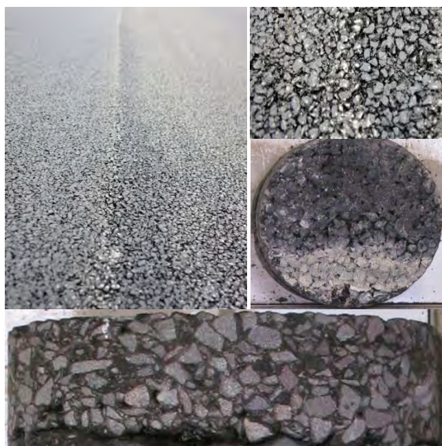
Figure 11: i) Photograph of joint C ii) Close up of joint iii) Surface of core 26 iii) Profile of core 26
