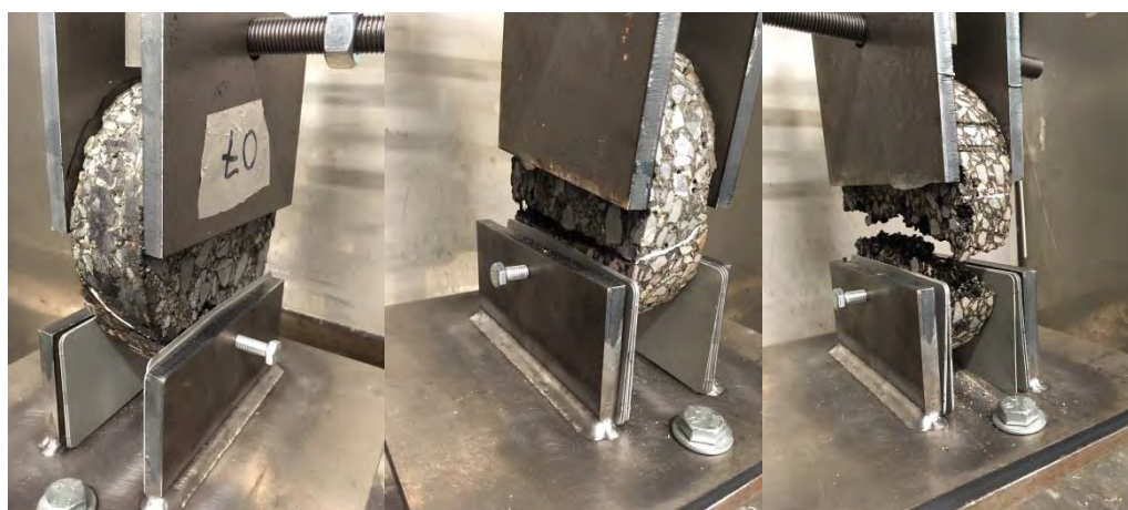
Figure 28: Photograph of test i) early test, started splitting, ii) testing just before failure iii) post test
