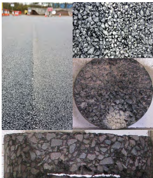
Figure 10: i) Photograph of joint B ii) Close up of joint iii) Surface of core 18 iii) Profile of core 18
