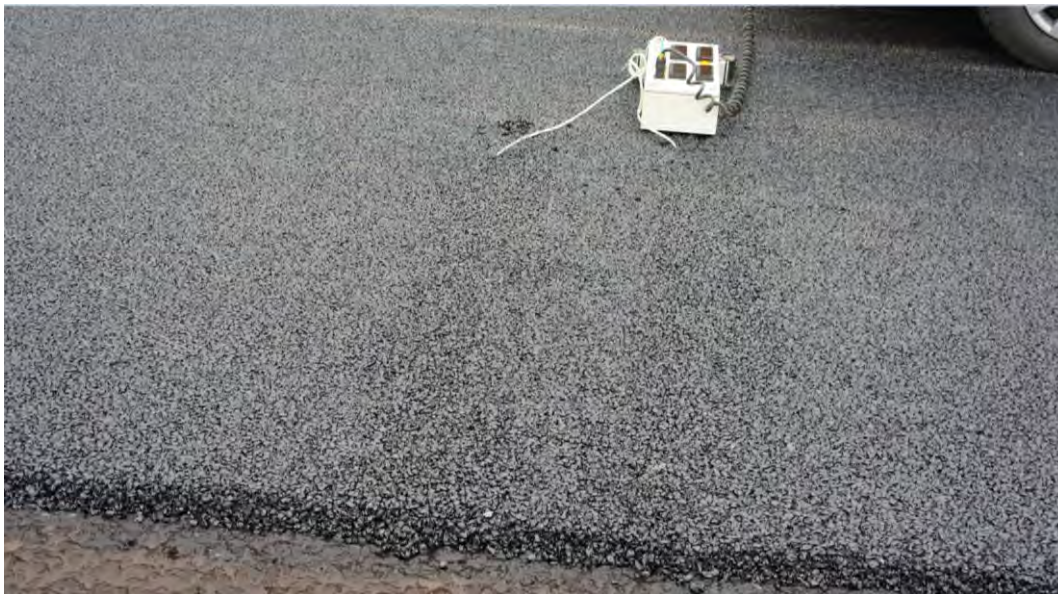
Figure 18: Installed thermocouples and data logger
