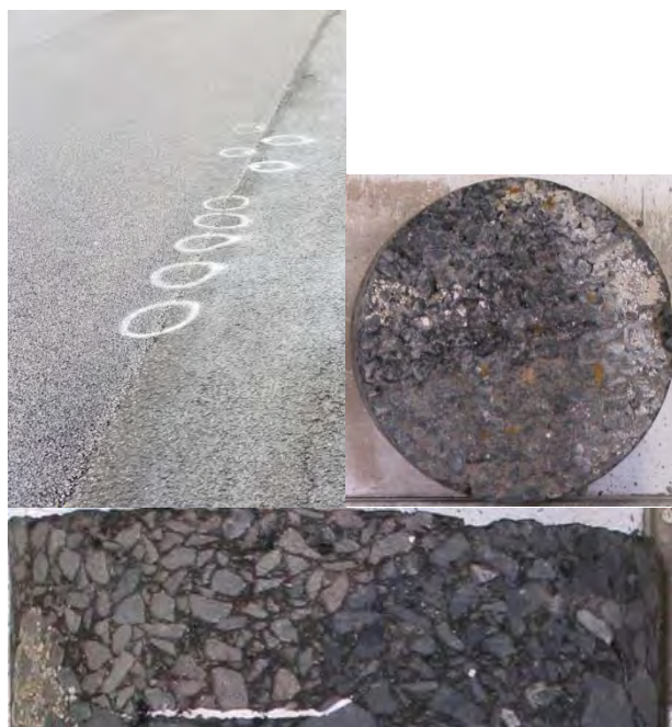
Figure 16: i) Photograph of the joint ii) Core 56 surface iii) Core 56 profile
