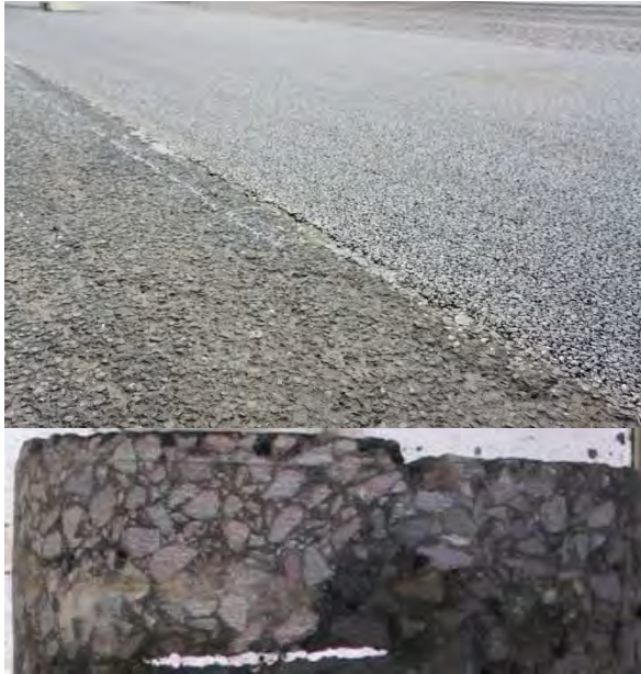
Figure 13: Painted Joint A; i) Photograph of the joint, ii) Core 8
