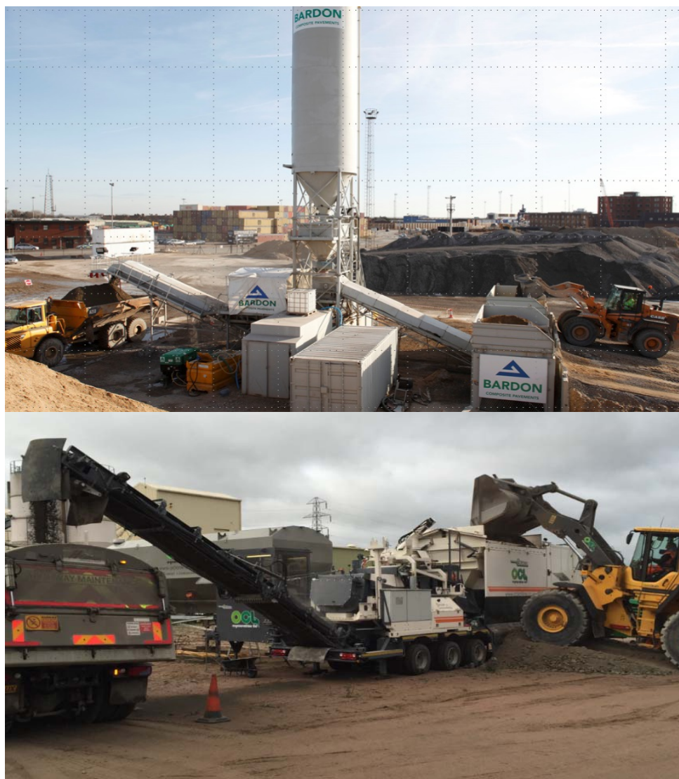
Figure 3 Typical production plant used for RCC (photographs courtesy of Aggregate Industries and OCL)
