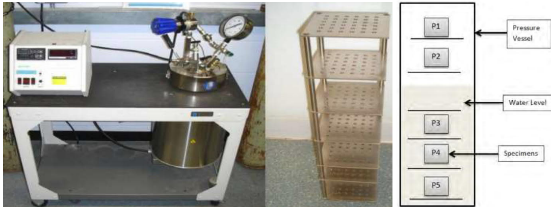
Figure 5. Modified SATS Test Equipment and Set-up (Ojum, Widyatmoko, Heslop, & Khojinian, 2017)
