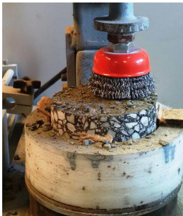
Figure 4. Modified Brushing Test (Thameside Test & Research Ltd, 2015)
