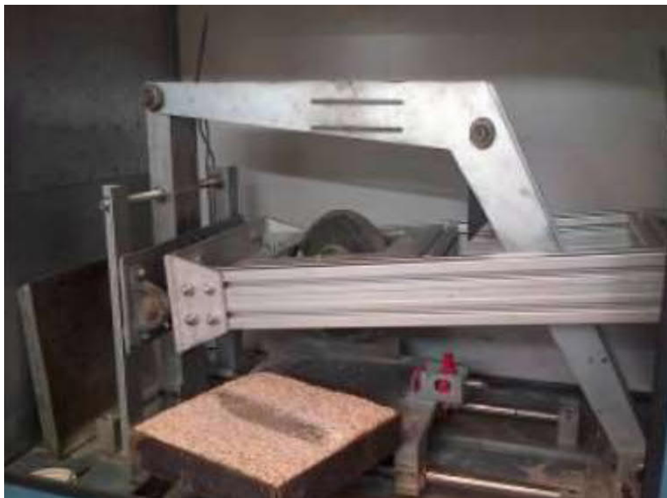
Figure 1. TRL Scuffing test (Ojum, 2016)
