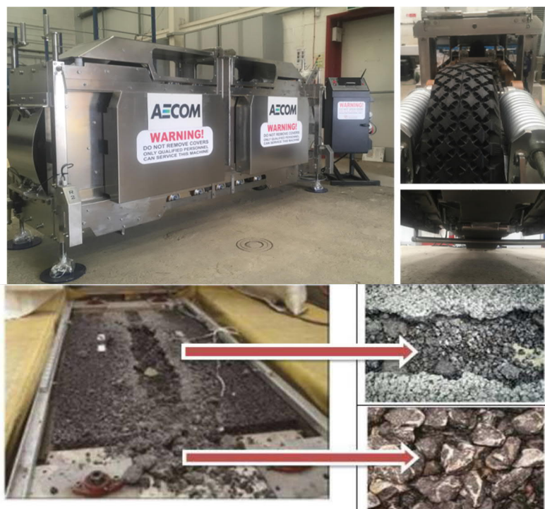
Figure 3. MLS 11 Equipment and Example of Stripping of Porous Asphalt tested with MMLS2 (Ojum, 2016)
