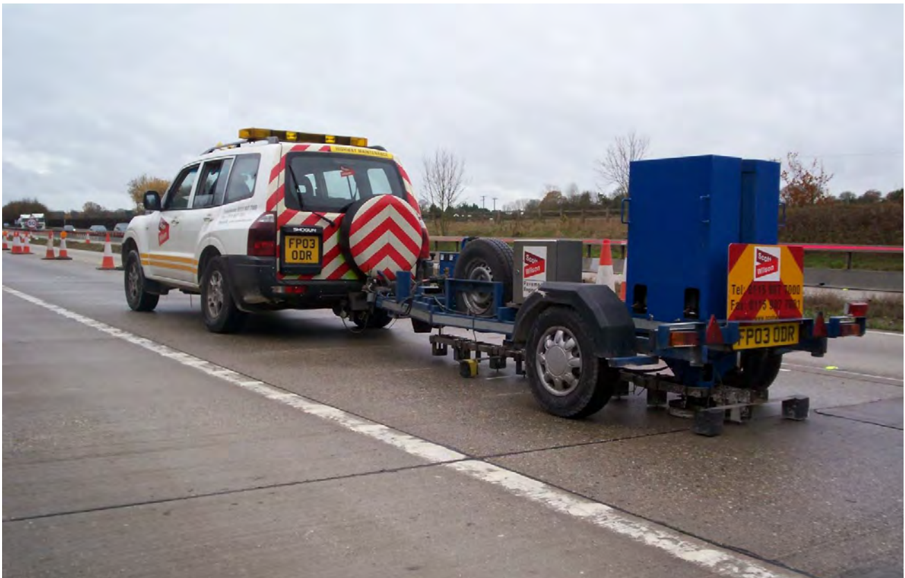
Figure 2.10 FWD undertaking concrete joint testing
