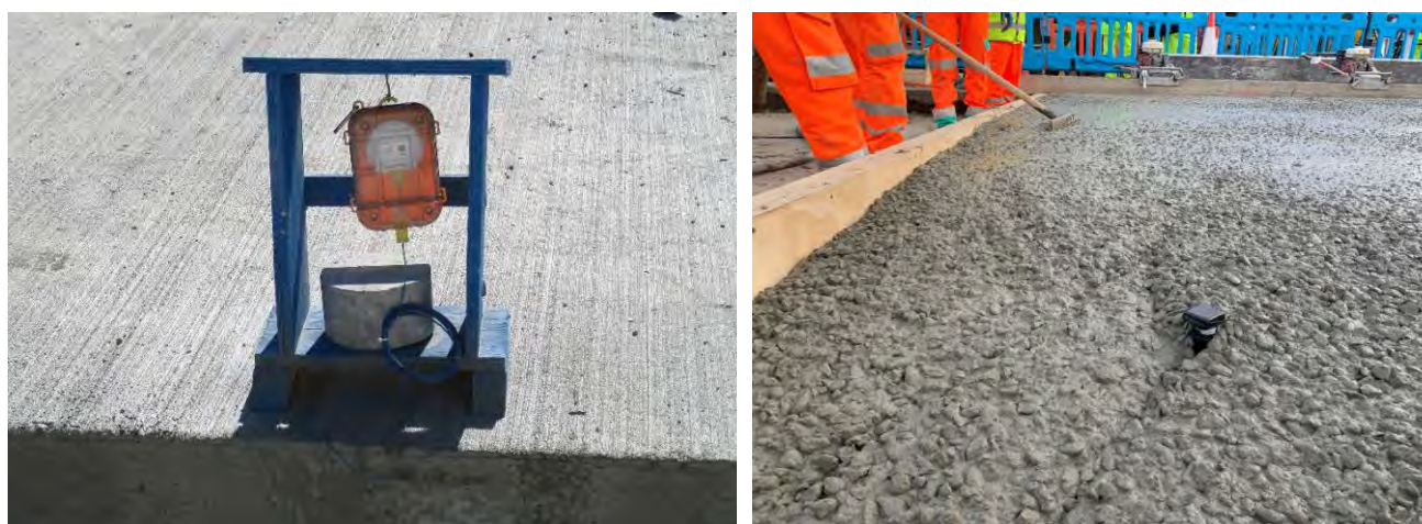
Figure 2.25 External transmitter with thermocouple placed in slab (left) and wireless sensor being installed within slab (right)
