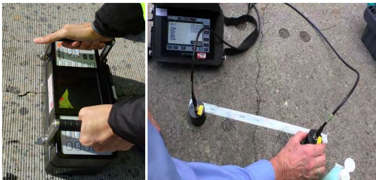
Figure 2.15 Ultrasonic tomography equipment [20]
