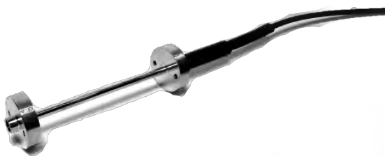
Figure 2.23 Fibre Bragg grating fibre optic sensor [34]
