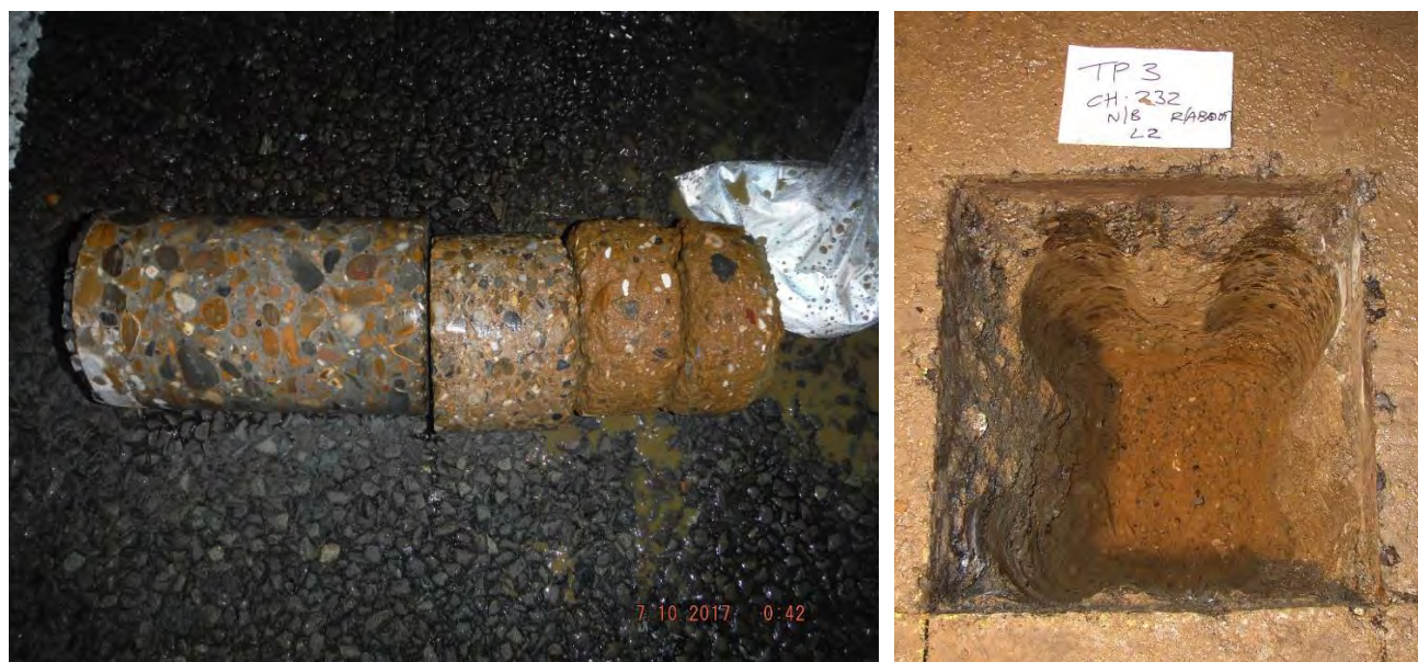
Figure 2.17 Extracted core (left) and multiple cores taken to create test pit (right)
