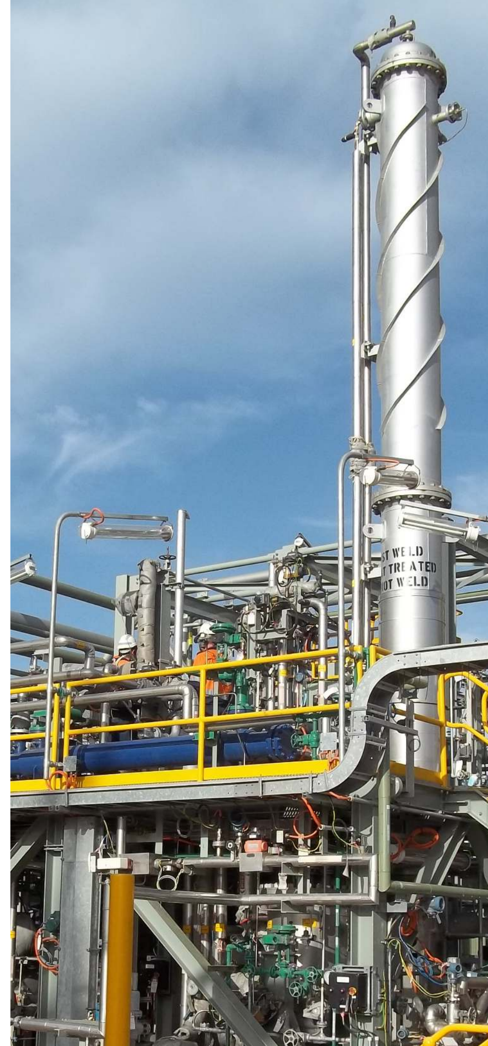
Photo right: Demonstration-scale CrystaSulf® unit in Australia removing H 2 S from a shale retort process gas stream.
