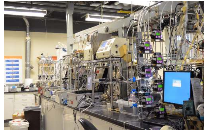
Trace metals and SO 2 chemistry is studied in a bench-scale FGD system.
