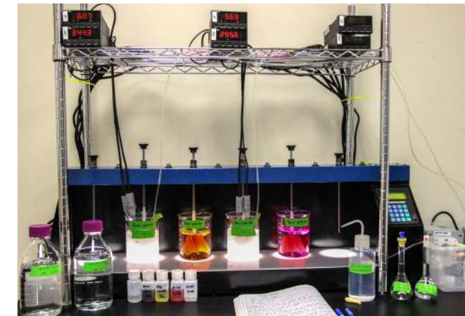
Jar testing apparatus equipped with pH controllers and ORP measurement capabilities to evaluate wastewater samples.
