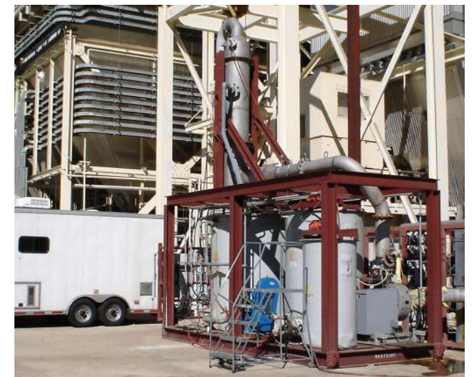
AECOM designed, fabricated and operated a pilot-scale system to evaluate the effectiveness of a limestone forced oxidized wet FGD process at removing catalytically oxidized mercury from flue gas.
