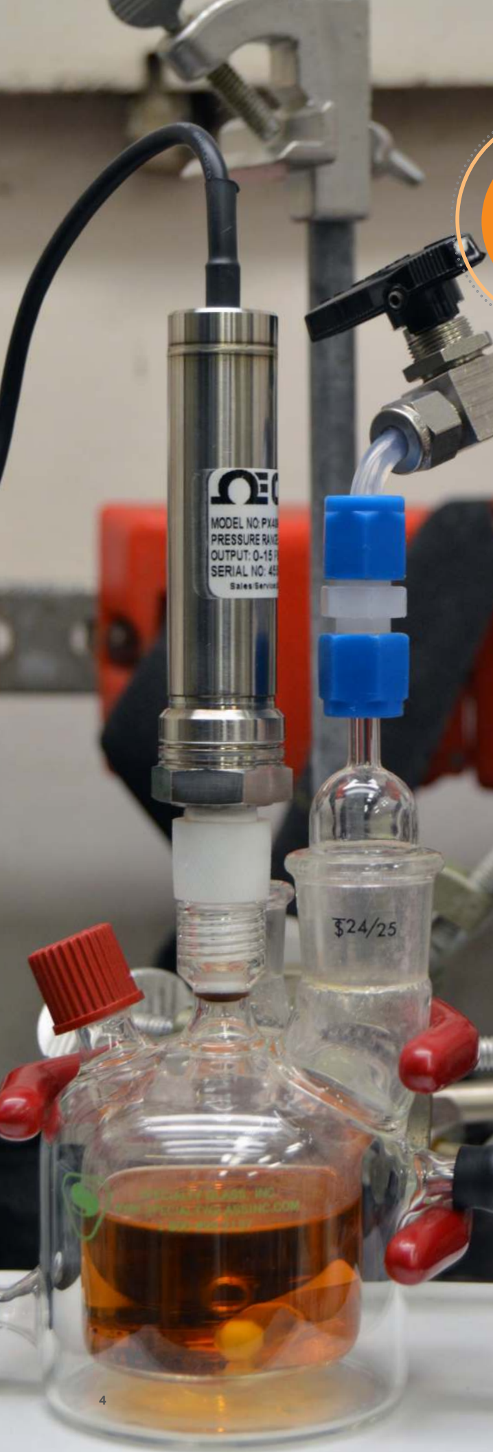
Photo left: Evaluation of an alternate solvent mixture for the CrystaSulf® H 2 S removal technology.
