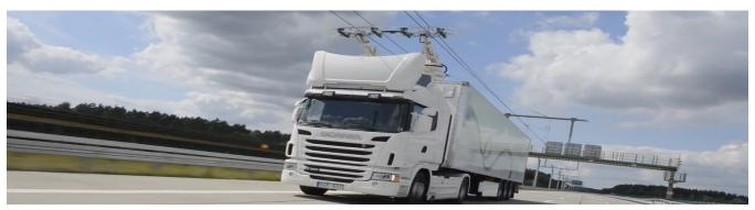
The E-Highway innovation supplies trucks with power from an overhead contact line. This means that not only is energy consumption cut in half but also local air pollution is reduced.
