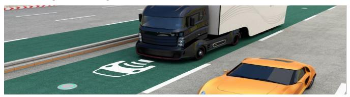
The growth of electric vehicles has been limited by motorists' concerns over vehicle range and charging infrastructure. AECOM is building a solution—inductive roadways that allow electric vehicles to charge as they drive.
