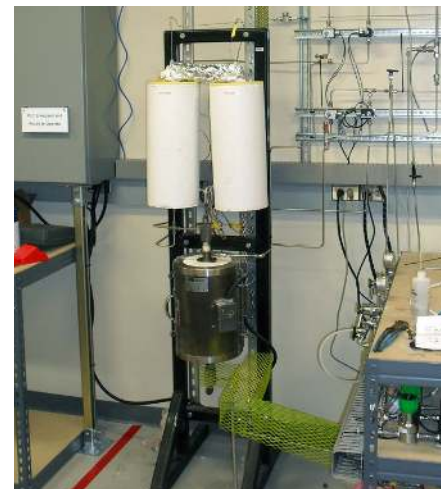
AECOM's High Temperature / High Pressure CO 2 Capture Laboratory Testing System.
