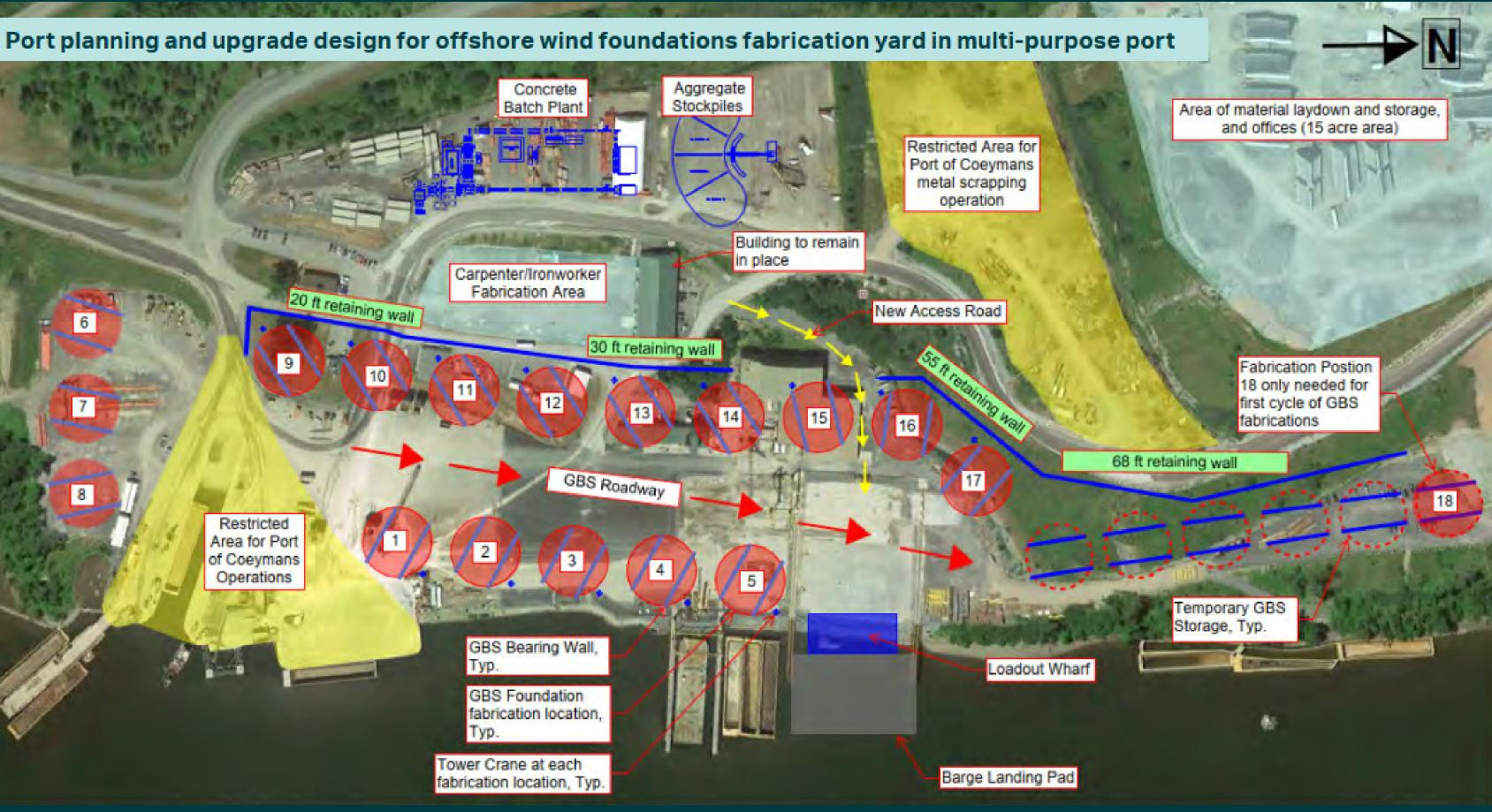
Develop site production layout with concrete batch plant Terminal modernization and infrastructure upgrades
