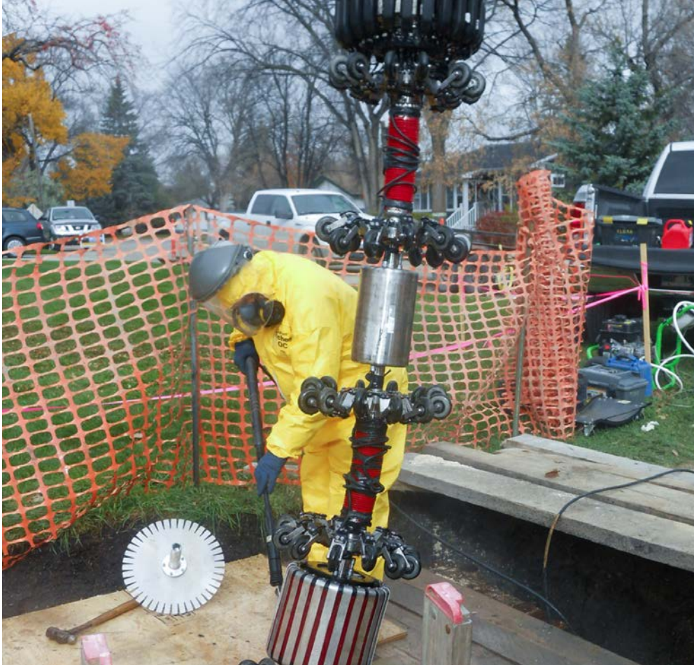
From left: High Risk River Crossing Management Program Winnipeg, Manitoba, Canada A remote field eddy current inspection platform was used in this City of Winnipeg program as a continuous assessment tool to identify remaining wall thickness and defect geometry of ferrous metal pipes.
