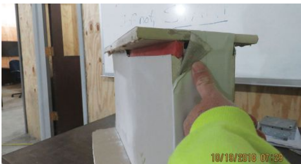
Mock-up for a head of wall when the bottom of the structure is the ceiling of the room. Corey Zussman photo
