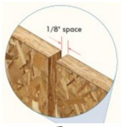
Roof H-Clips may not create the 1/8" movement gap...make sure that there is an 1/8" gap horizontally.
