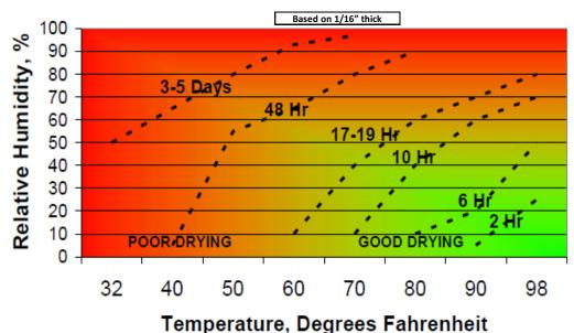
Graph Reference – The color-coded graph provides an easy-to-interpret map of joint compound
