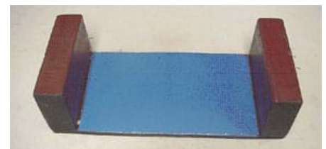
Figure 5. Wooden support structure for the testing station. Blue represents the water below the bridge. The end blocks represent bridge abutments.
