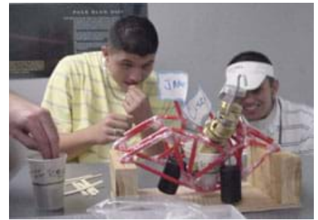
Figure 9. This straw bridge was so strong that it took more than a cup of pennies to make it collapse.
